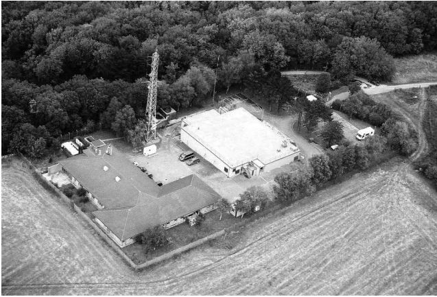
Figure 2.6 The anti-aircraft operations room at Lansdown, west of Bristol. The square block house (centre) is the semi-sunken protected control for gun defended area two until 1956.
