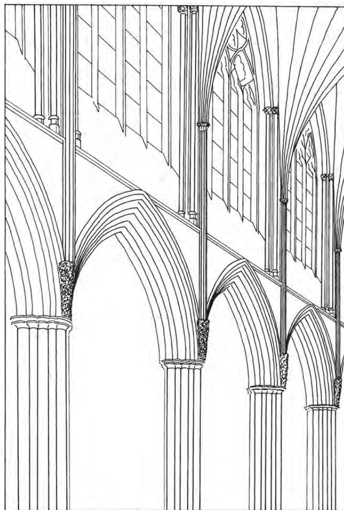
Fig. 8. Exeter Cathedral, reconstruction of original form of presbytery elevation (drawing by Christopher Wilson).
