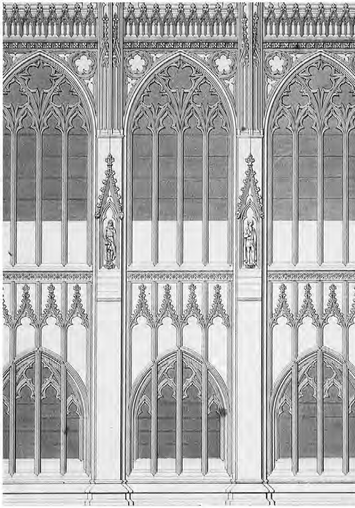
Fig. 7. Westminster Palace, St Stephen's Chapel, part of south exterior elevation: upper chapel windows shown with hypothetically reconstructed tracery and later blocking in lower parts of lights (from F. Machenzie, The Architectural Antiquities of the Collegiate Church of St Stephen, Westminster , London, 1844, detail of Plate IV).
